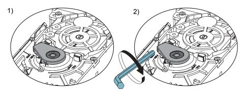
d When stop arm is on the bottom of the operator, loose the stop arm locator and the stop arm. Mount the stop arm on the splines, as close as possible to the stop block 3). Mount the stop arm locator. Fine-adjust if necessary with the screw on the stop arm 4).
