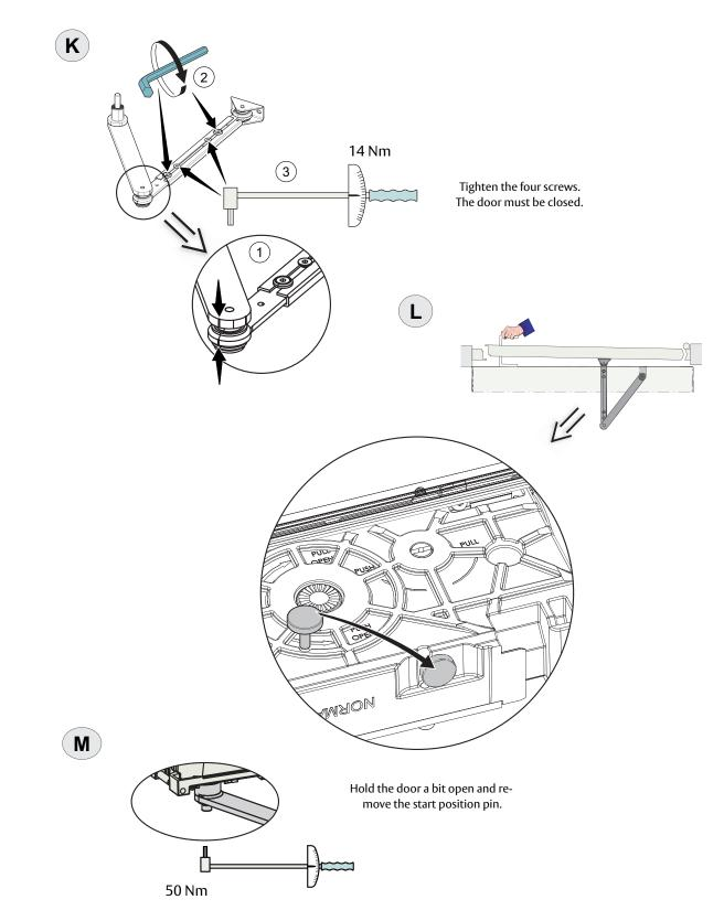
Note! Important to make sure you tighten with 50 Nm before finalizing the mechanical installation! See the table on page 27 for available extensions. Continue on page 63.
