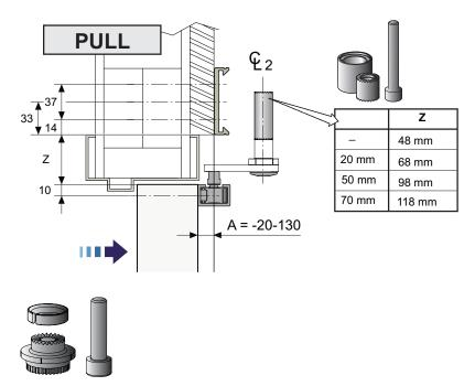
**Note!** Measurement Z must be reduced by 20 mm if lower adapter from kit DAB805LA is used.
