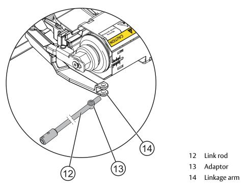
j Mount on the other side of the link rod (12) to the secondary motor unit with the signal (16). Fasten the stop screw (17).
