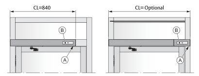
(A) Reset & Indication device (B) Smoke detector
