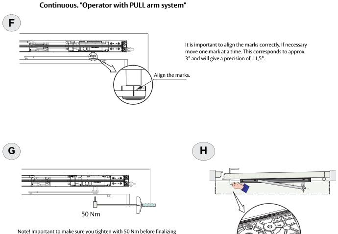
Note! Important to make sure you tighten with 50 Nm before finalizing the mechanical installation!
