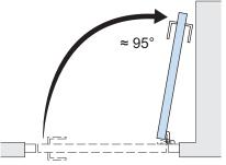
c When stop arm is on top of the operator, lift the door stop arm up and mount it on the splines, as close as possible to the stop block 1). Fine-adjust if necessary with the screw on the stop arm 2).
