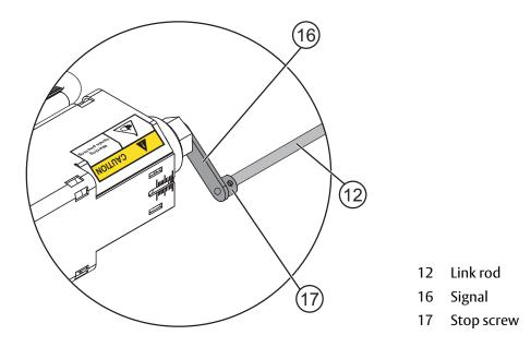
k Adjust the release of the brake by loosening the joint (18) and turning the link rod (12) close to the primary drive unit. Make the angle between the doors near closed position.
