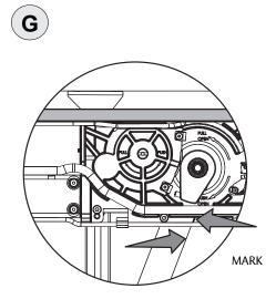
Align the arm with the operator mark.
