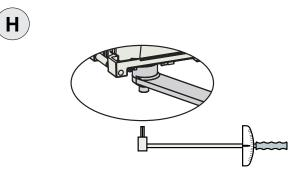
Tighten the screw temporary to keep the arm in place.
